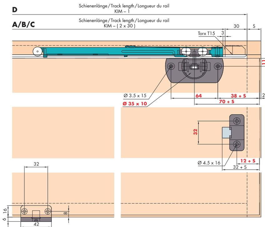
Türbearbeitung = rote Zahlen / Dimensions and drillings for doors = red numbers / Usinage de la porte = chiffres rouges
