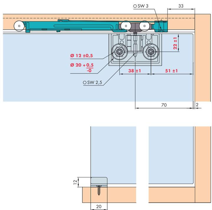
**Türbearbeitung = rote Zahlen/Dimensions and drillings for doors = red numbers/Usinage de la porte = chiffres rouges**
