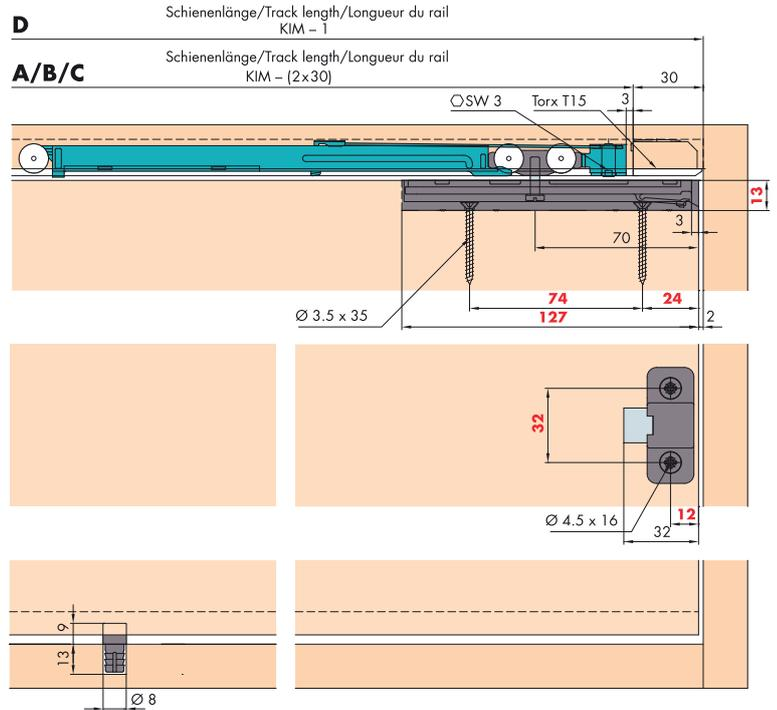
Türbearbeitung = rote Zahlen/Dimensions and drillings for doors = red numbers/Usage de la porte = chiffres rouges
