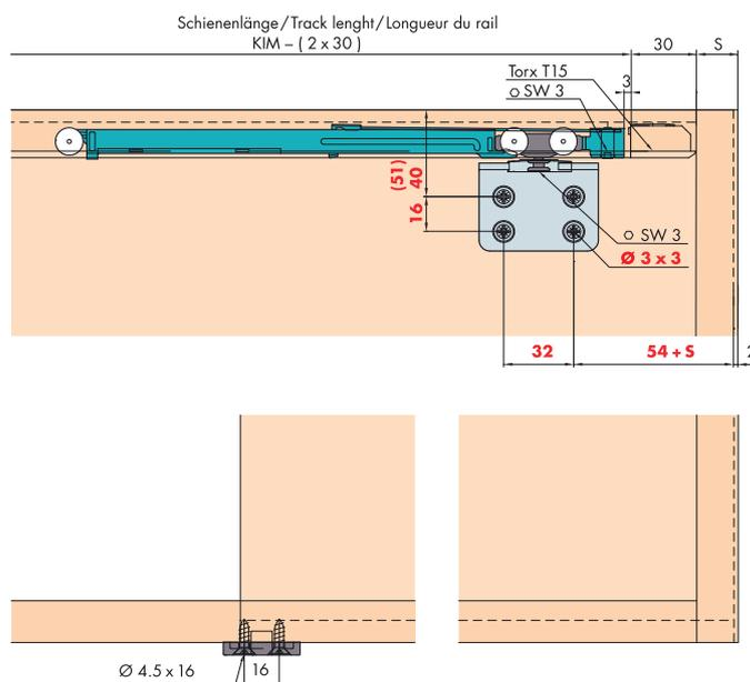
**Türbearbeitung = rote Zahlen/Dimensions and drillings for doors = red numbers/Usinage de la porte = chiffres rouges**
