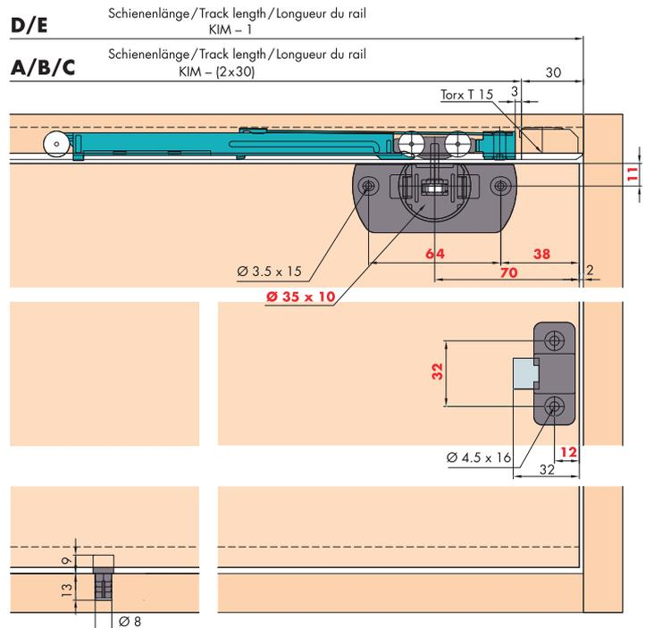
**Türbearbeitung = rote Zahlen/Dimensions and drillings for doors = red numbers/Usinage de la porte = chiffres rouges**
