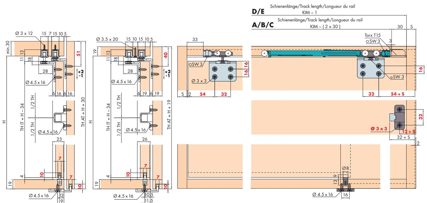
Türbearbeitung = rote Zahlen/Dimensions and drillings for doors = red numbers/Usinage de la porte = chiffres rouges
