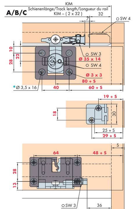
Türbearbeitung = rote Zahlen/Dimensions and drillings for doors = red numbers/Usinage de la porte = chiffres rouges
