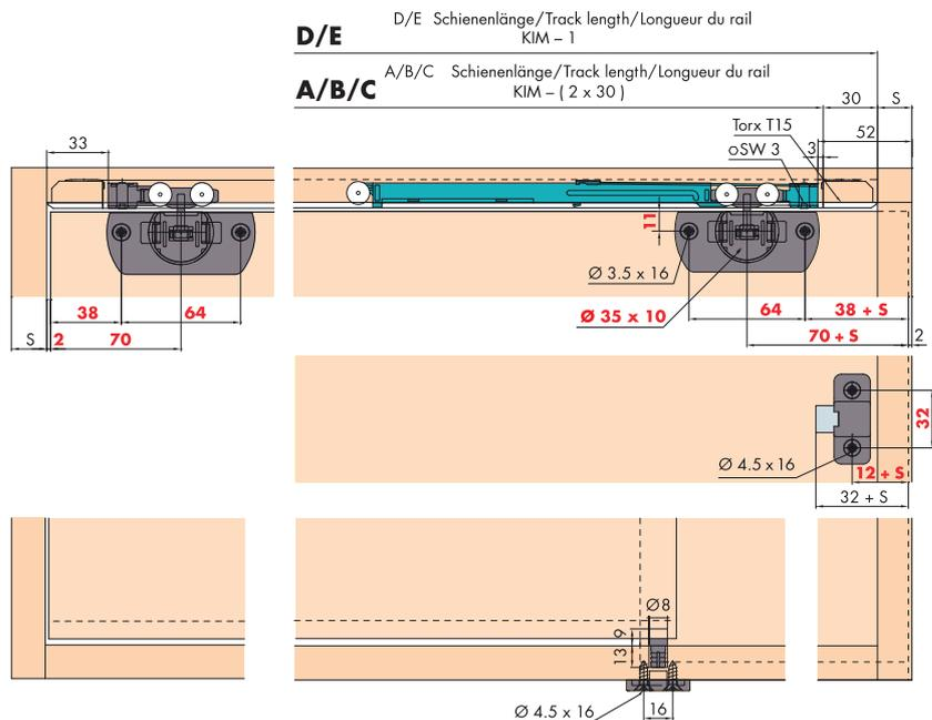
Türbearbeitung = rote Zahlen/Dimensions and drillings for doors = red numbers/Usinage de la porte = chiffres rouges
